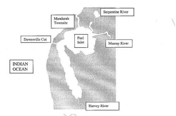
In 1995 the Dawesville Cut was completed south of Mandurah. This is a deep channel joining the inlet to the ocean. As a result the inlet waters are extensively flushed by the rise and fall of the tides and the waters of the inlet are circulated more effectively.
